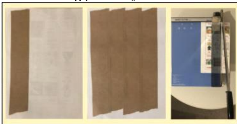
FIGURE 3. How to Apply the Backing to Reduce Waste
